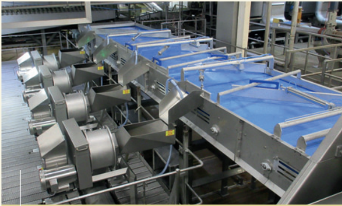
Four Tridis 240P machines integrated in a high capacity French fry production line.
