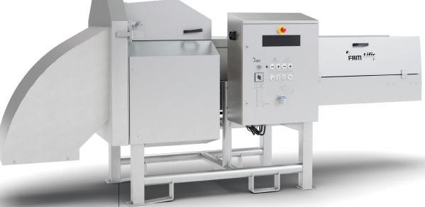
The Lifis.2 can be supplied with a large number of interchangeable cutting wheels offering maximum flexibility in cut sizes and types (flat slice, crinkle slice, square pieces etc.).
